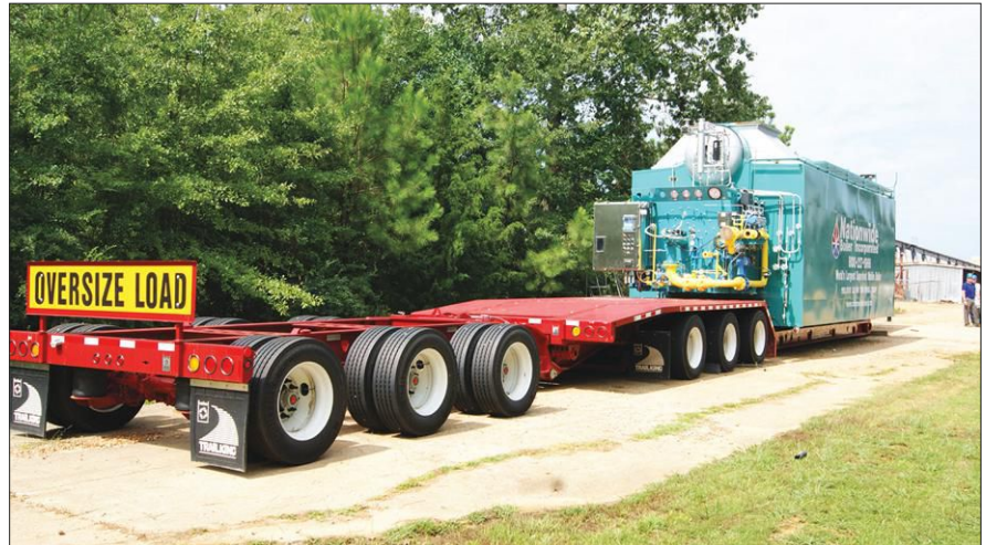
FIGURE 2. A 110,000-pound-per-hour, trailer-mounted, rental boiler – the “world’s largest” mobile, superheated steam boiler.
