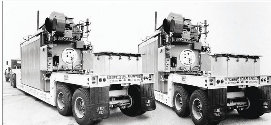
FIGURE 6. Some of the first 20,000-pph, trailer-mounted rental boilers were developed 55 years ago by Nationwide Boiler in 1967.
