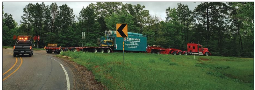
FIGURE 3. A 125,000-pound-per-hour, trailer-mounted, rental boiler – the “world’s largest” mobile, saturated steam boiler.
