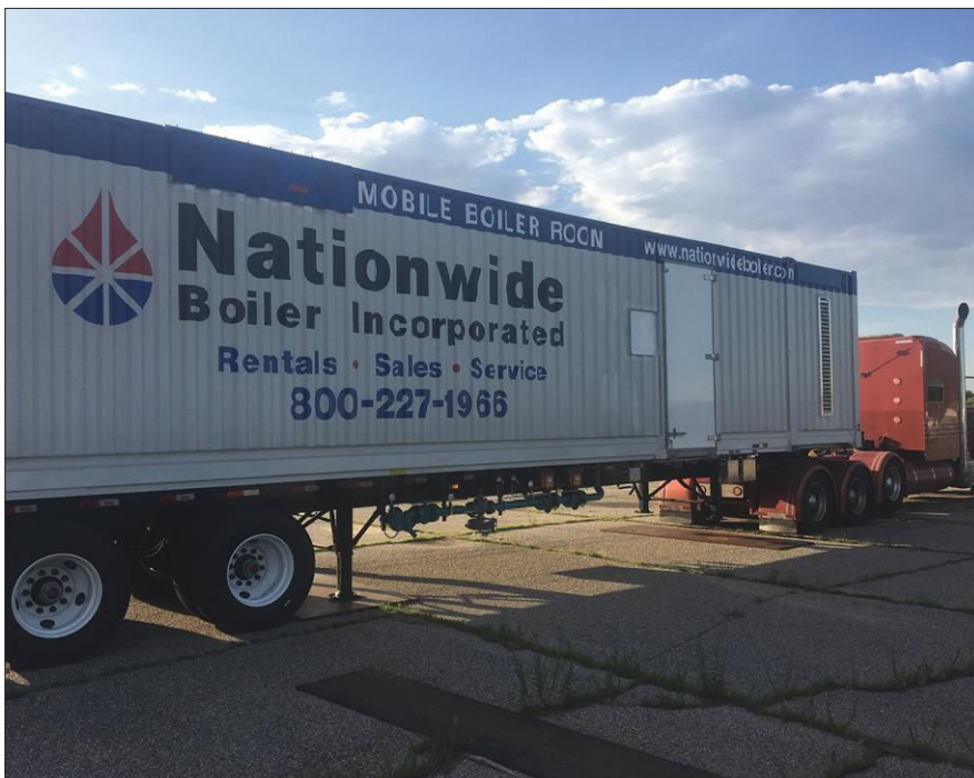
FIGURE 4. A 1,000-hp mobile boiler room hooked up to a tractor-trailer for transit to its next rental project.
