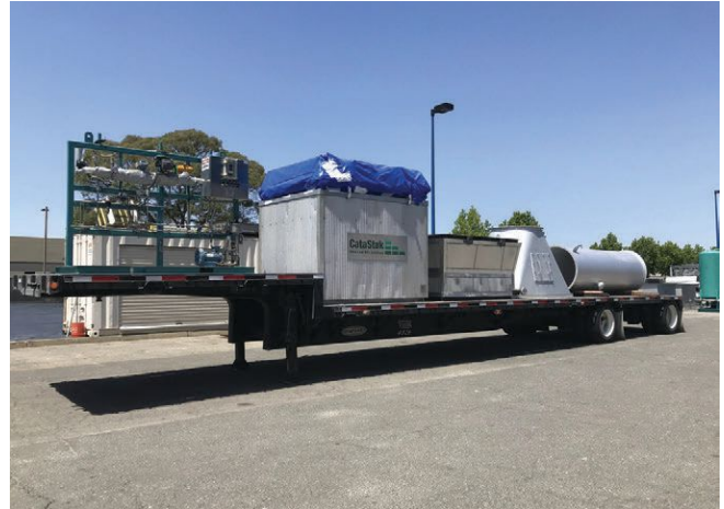
A flatbed shipment with all the temporary SCR system components that are typically provided by the rental supplier.
