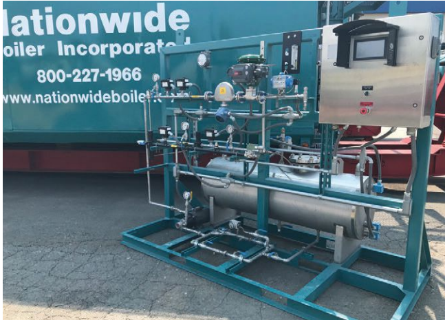
A urea supply skid for a temporary SCR system.
