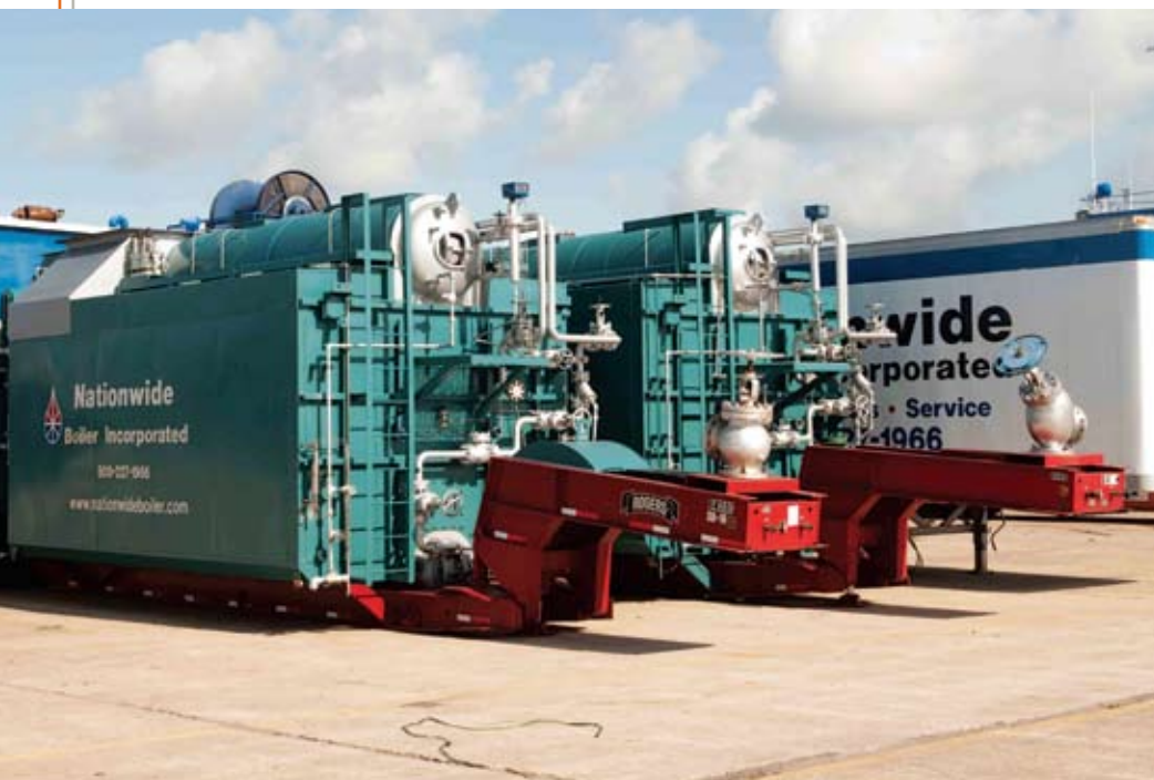
FIGURE 2. TWO 70,000 LB/HR TRAILER-MOUNTED BOILERS AND ONE 140,000 LB/HR MOBILE FEED-WATER VAN.
