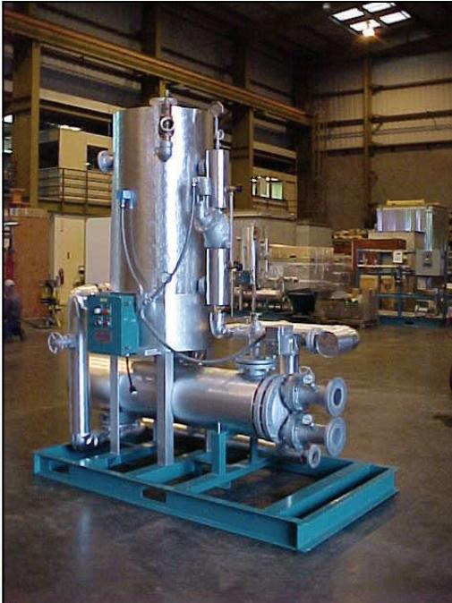
Why waste valuable energy through continuous surface blowdown when it can be recovered to preheat boiler feedwater? The Nationwide Boiler Heat Recovery (HR) Blowdown Pac has been developed to increase efficiency up to 2% and can offer significant savings in fuel and operating costs with a quick return on investment. Often times end users can see dramatic energy savings in less than one year, as well as increased efficiencies.
