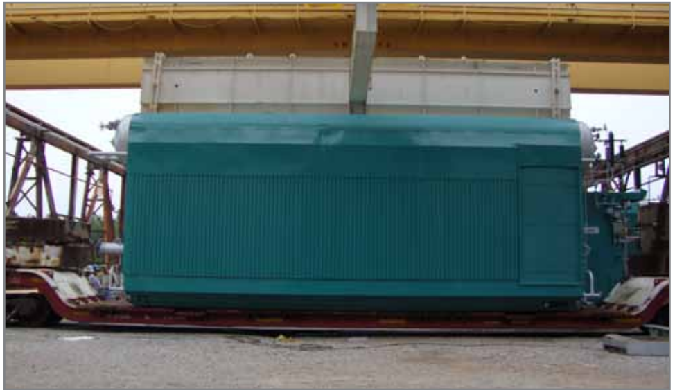
New Babcock & Wilcox 200,000 lb/hr watertube boiler being loaded for shipment to Mexico by rail.
