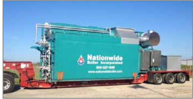
New 70,000 lb/hr Nebraska Trailer-mounted boiler on route to Westlake, Louisiana
