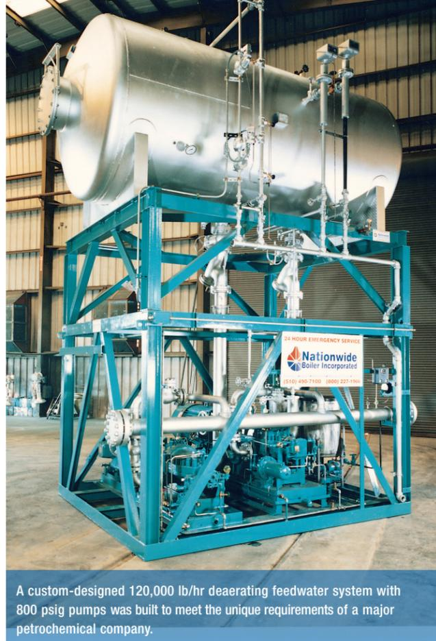
A custom-designed 120,000 lb/hr deaerating feedwater system with 800 psig pumps was built to meet the unique requirements of a major petrochemical company.
