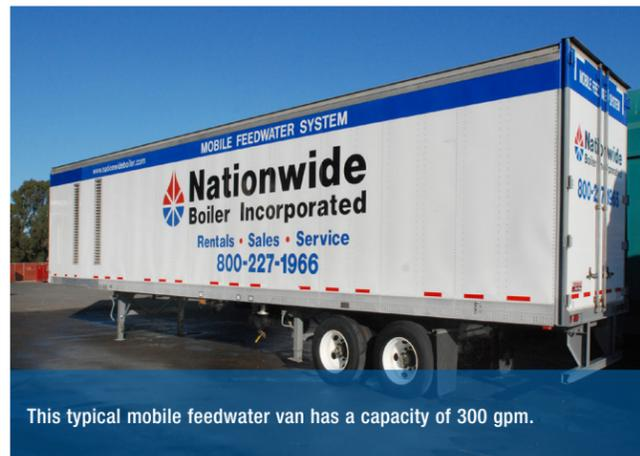
This typical mobile feedwater van has a capacity of 300 gpm.
