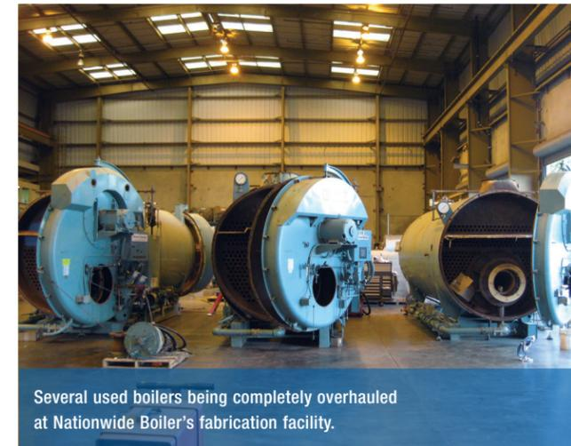
Several used boilers being completely overhauled at Nationwide Boiler's fabrication facility.
