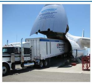
Nationwide Boiler supplied Kentz Qatar with two 70,000 lb/hr trailer-mounted rental boilers and one 140,000 lb/hr mobile feedwater van to accomplish the task at hand. The equipment was loaded on the Mignon ro-ro ship (roll on/roll off) at the Port of Galveston, TX and was in transit for over thirty days before reaching the Doha Port.
