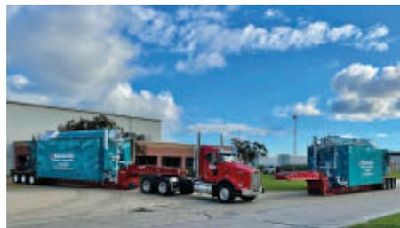
Two Nationwide Boiler 75,000 lbs/hr trailer-mounted, superheated steam rental boilers
