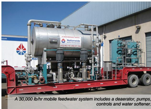
*A 30,000 lb/hr mobile feedwater system includes a deaerator, pumps, controls and water softener.*
