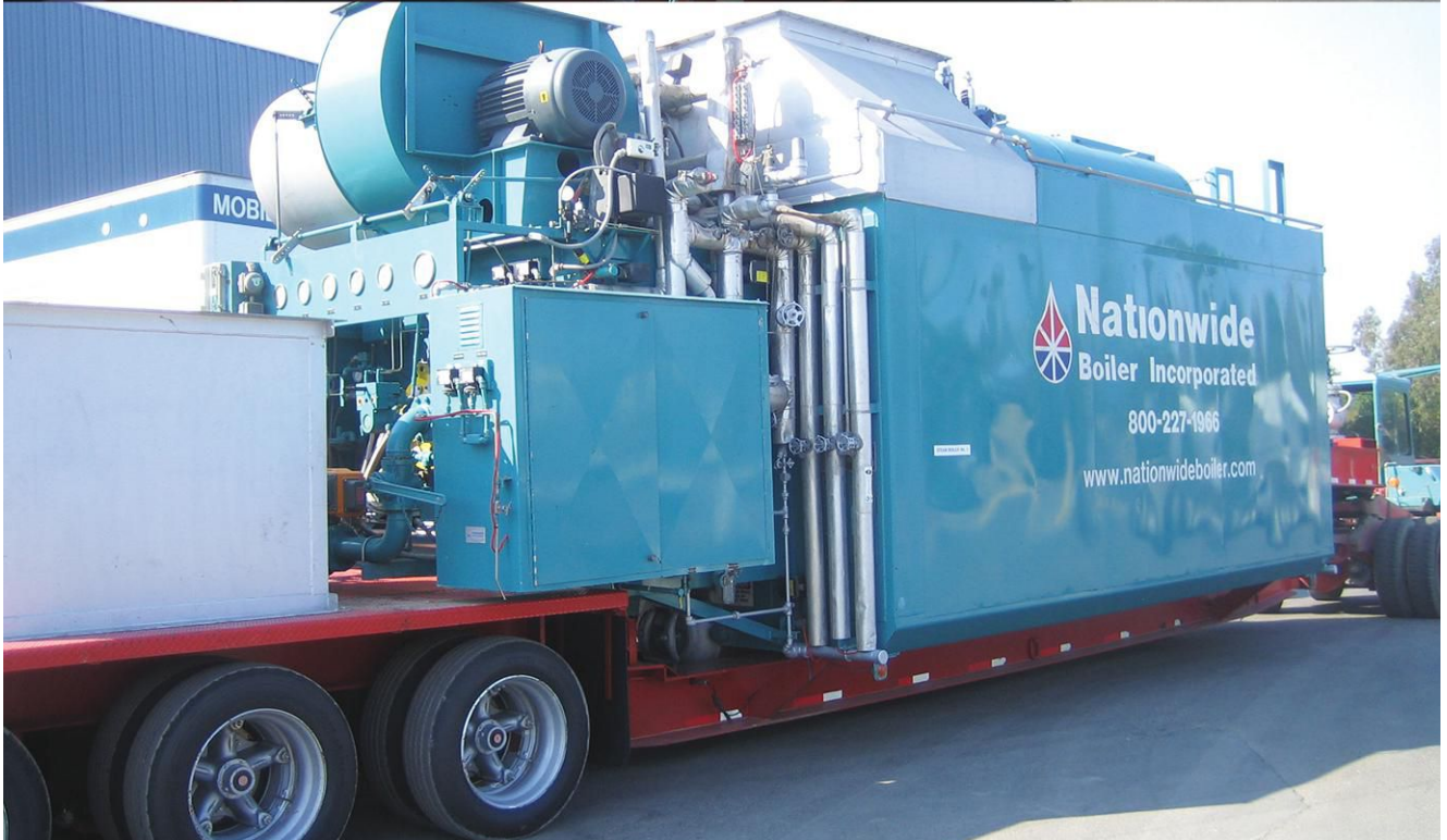
This trailer-mounted watertube rental boiler with heat tracing and insulation is properly protected from the elements.
