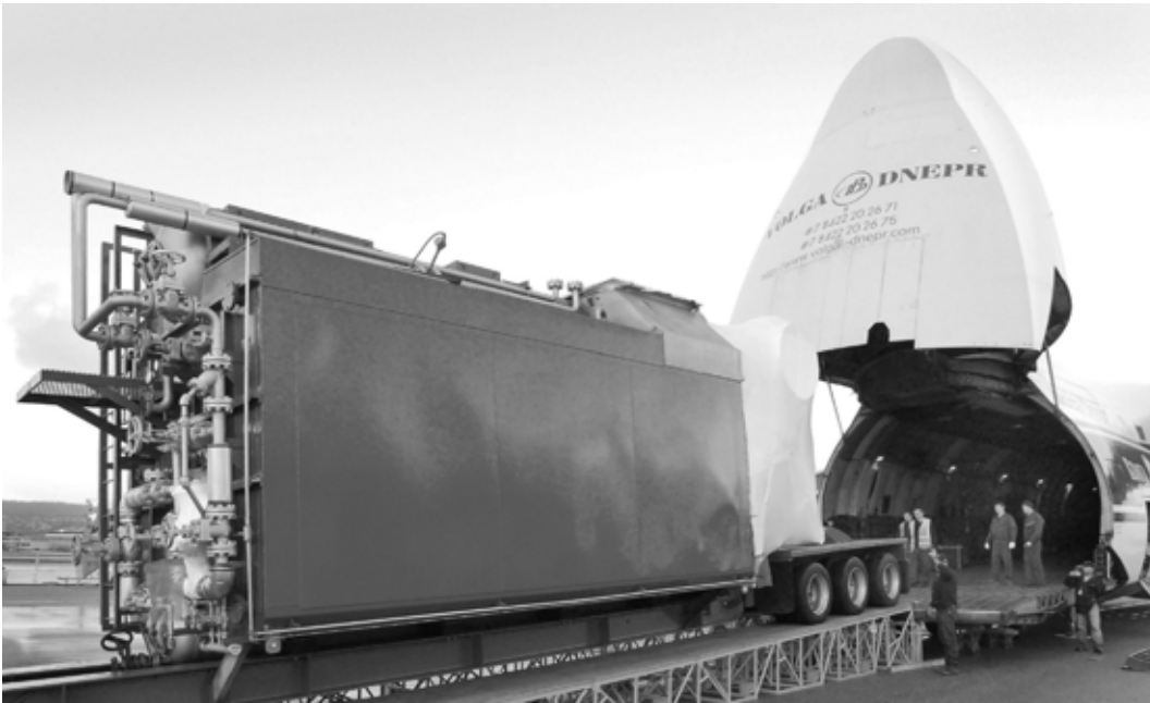
70,000 pph trailer-mounted boiler being loaded into the Antonov AN124-100 at San Francisco International Airport
