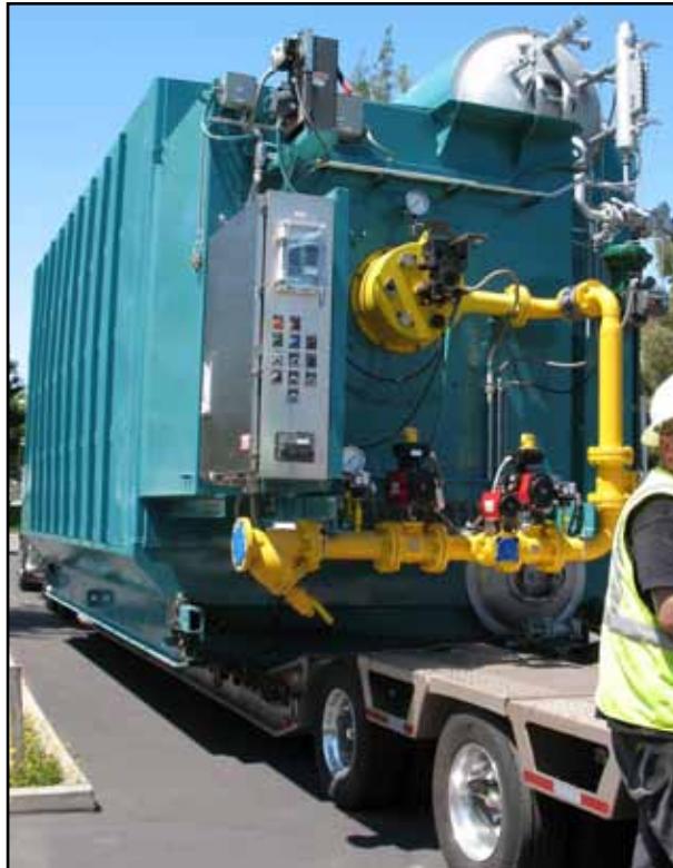
Reconditioned 70,000 lb/hr skid-mounted Nebraska "D" type boiler sold to SUG as a replacement boiler.
