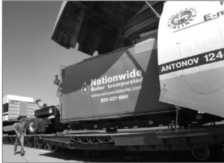
70,000 pph trailer-mounted rental boiler being loaded onto the Antonov Aircraft for delivery to Qatar.
