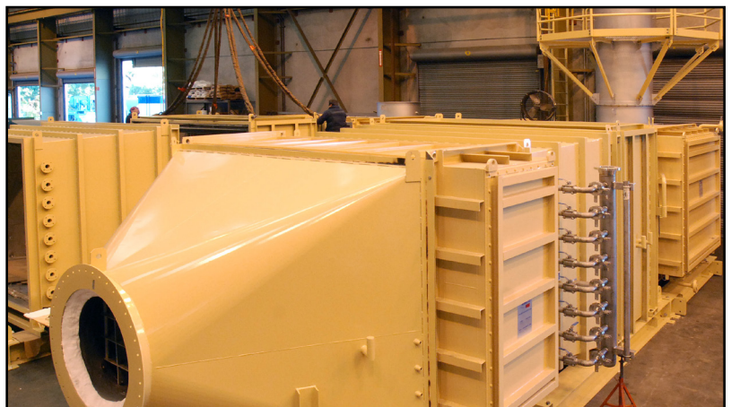
Two (2) CataStak™ SCR Systems for Allison 501 4MW Turbines Used for 1200 psi Down Hole Steam Injection
